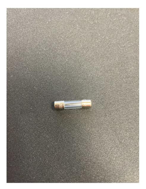
**7. Replace the fuse:** If the fuse is blown or damaged, it needs to be replaced. If you have the extra fuses that came with your chair, take one of the T5AL250V Cartridge Glass Fuses and insert it into the empty fuse holder, aligning the metal ends correctly.
